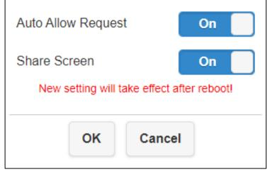
5.4.1 Auto Allow Request: Once turned on, all the connecting devices can cast without the host transmitters approval.
